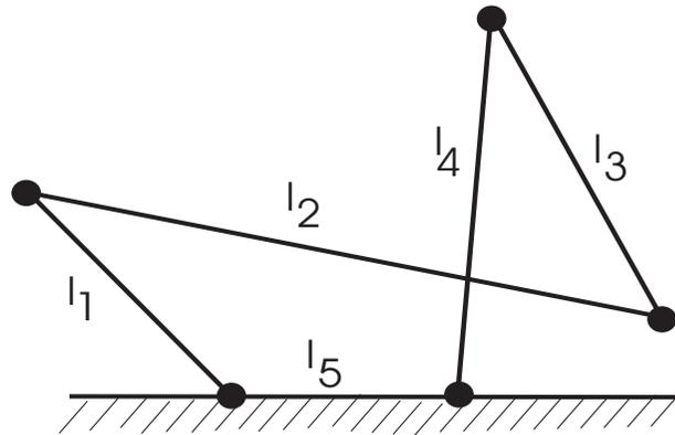
A planar linkage is a mechanism consisting of  $n$  bars of fixed lengths  $l_1, \dots, l_n$  connected by revolving joints forming a closed polygonal chain. The positions of two adjacent vertices are fixed but the other vertices are free to move so that angles between the bars change but the lengths of the bars remain fixed and the links are not disconnected from each other.
